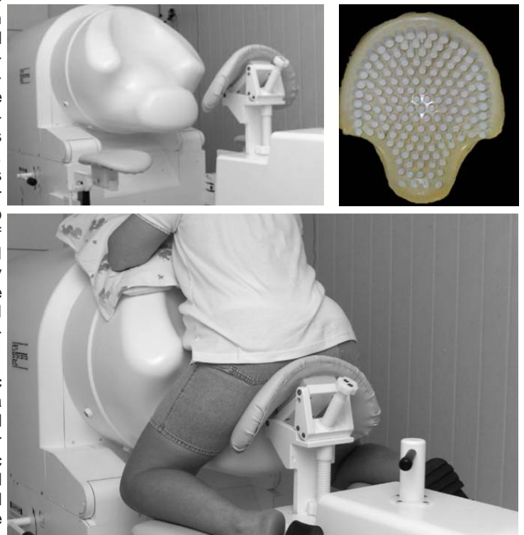
Figure 1. SARA, consisting of 151 gradiometers arranged to comfortably fit the gravid abdomen.
