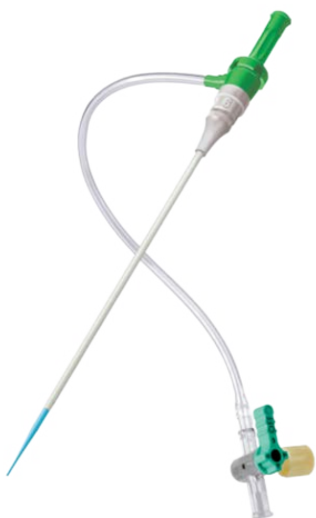
FIGURE 2 Terumo Slender Glidesheath for Radial Artery Access This is a 6Fr Slender Glidesheath (Terumo Interventional Systems, Somerset, NJ). It has a 2.44 mm outer diameter compared to a regular 6Fr sheath with an outer diameter of 2.63 mm. It has a thin wall that allows for a better sheath to radial artery diameter ratio, which reduces spasm and radial artery occlusion, but it does make the sheath easier to kink.
