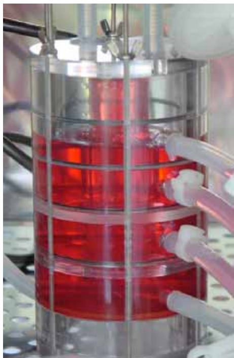
Figure 4. "Bioreactor" system developed by the Jockenhoevel group for mechanical conditioning of autologous heart valves prior to implantation.
